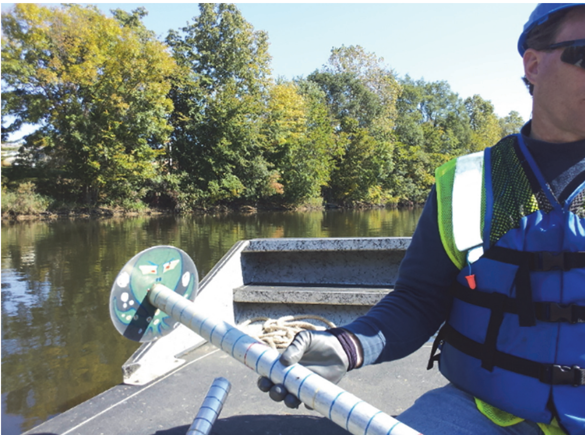
Figure 3-11—Poling to Detect Sunken Oil in the Kalamazoo River (F. Fitzpatrick, USGS)
