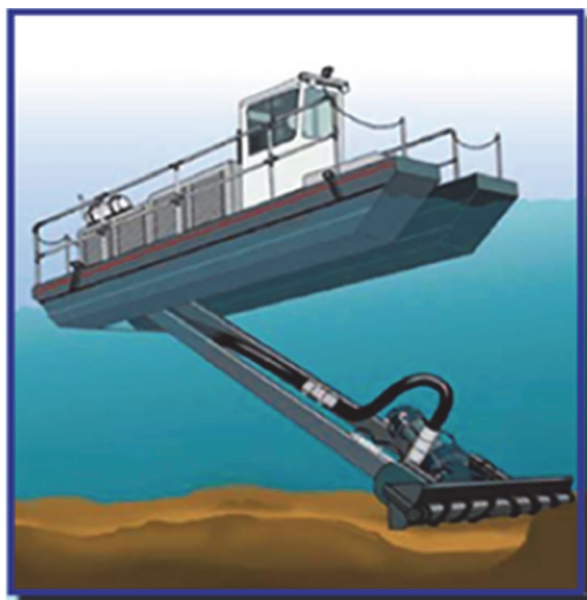
Figure 5-1—Portable Suction Dredge with Cutter/auger Head Similar to the One Used in the T/B Morris J. Berman Response (SRS Crisafulli, Inc., Glendive, Montana)
