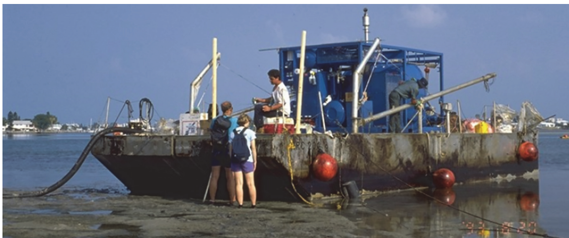
Figure 5-5—Portable Vacuum Transfer Unit (VTU) Mounted on a Portable Barge During the 1993 T/B Bouchard 155 Incident (NOAA)
