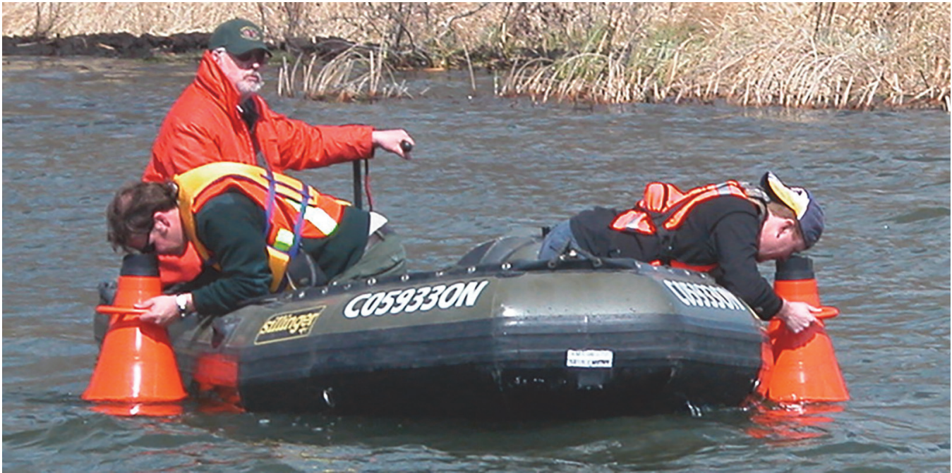
Figure 3-8—Sunken Oil Detection Using Underwater Viewers at Lake Wabamun (E. Owens, OCC)
