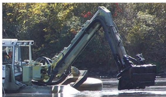
Figure 5-2—Amphibious Suction Dredge Used On the Enbridge Pipeline Response in the Kalamazoo River ( www.enbridge.com )
