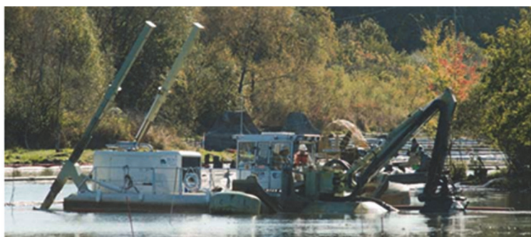
Figure 5-2—Amphibious Suction Dredge Used On the Enbridge Pipeline Response in the Kalamazoo River ( www.enbridge.com )
